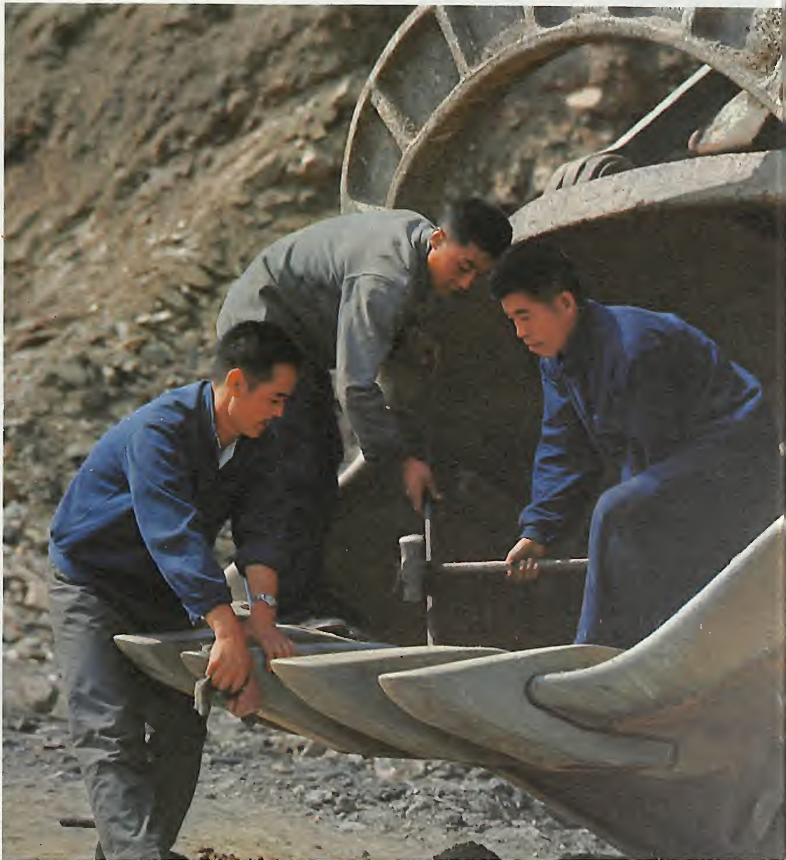
Drivers of drilling machines, power shovels and trucks coordinate closely. Here they are overhauling a power shovel.
